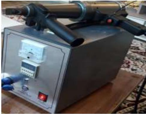
Figure 3: Ultrasonic peening device type HC-S-1
