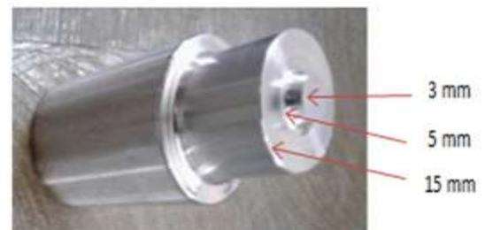
**Figure 2:** Cylindrical tapered Pin Tool
