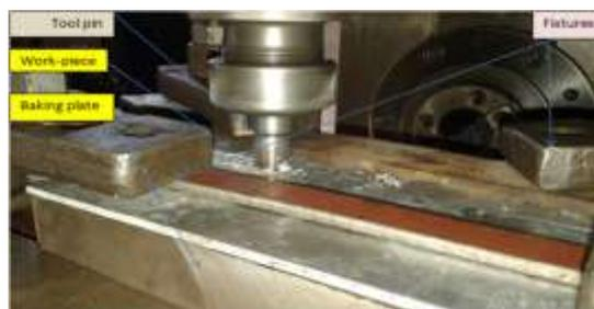
**Figure 1:** Milling Machine and Fixture System
