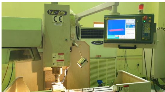
Figure 1: 3-Axis CNC milling machine "C-tek" type
