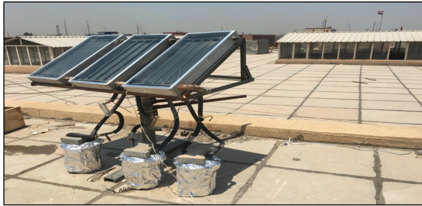
Figure 1: Schematic of flat-plate solar collector
