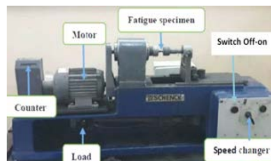
Figure 2: Fatigue rotating bending machine (SCHENCK PUNN).
